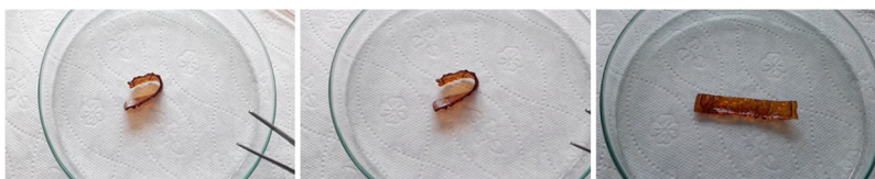
Figure 7. Representative shape memory performance of cured PGL 20 M 80 I copolyester samples at room temperature.
